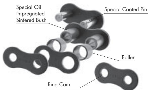
Fig. 31 Basic Construction
